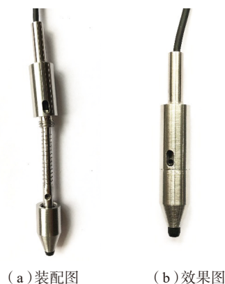
图4 机械自补偿涡流探头装配效果图 Fig.4 Eddy current probe of mechanical self-compensation
